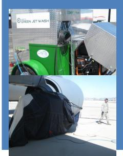
Collection suit is the only system in the world that collects <u>ALL</u> the effluent coming out of the tail pipe and engine while performing engine compressor wash. This system encapsulates the engine. There is a screened vent on top of the suit to allow excess air to escape the suit to prevent over inflation of the suit. The material this suit is made of is of a space age fabric which is extremely light and durable and has proved to be ideal for its purpose. This suit conveniently fits in a
